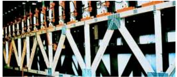
Laboratory Testing of Wood Trusses
